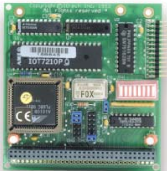
Personal488/MM converts any PC/104 embedded PC into an IEEE 488.2 controller
